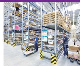
shelving has a negative impact on pick time. A third solution involves static shelving parallel to racking, which makes front items easy to pick. Shelving dividers can be fitted.
