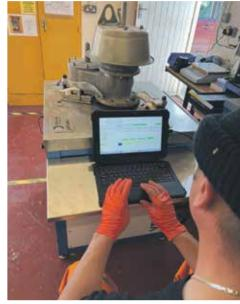
The testing of breather valves, both when new and during their service life, is crucial. The testing equipment should meet the following criteria as per API2000 Section 5.4:
