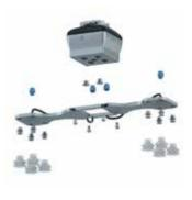
The VGC10 gripper has a customised fixture with 4 suction cups and is programmed to handle 2 rollers at a time to match the production cycle.
