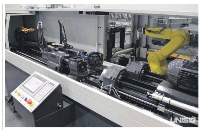
pallet. Where a part is gripped impacts where it is clamped for drilling to ensure accuracy. Every variable along the process chain must be considered and accounted for, and the calculus is detailed and complicated.
