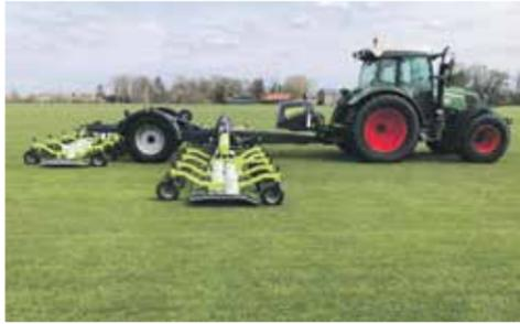
The Eco Clipper® Mowing System offers many advantages over traditional cylinder and rotary mowers. Because it consists of an independently suspended 106cm wide deck section, it is cleverly linked together in larger, flexible contour following mowing decks. The entire design and development of the Eco Clipper® Mowing System delivers a clean cut, even clippings dispersion and excellent following of the ground contours with minimal soil compaction.
