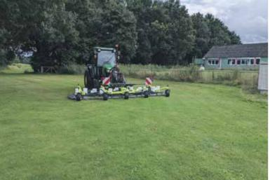
The smooth cutting decks with fast rotating small blades ensure a high quality of cut and a good distribution of the clippings. The clippings are also well spread in wet grass, which makes it possible to schedule the mower almost independently to all weather conditions.
