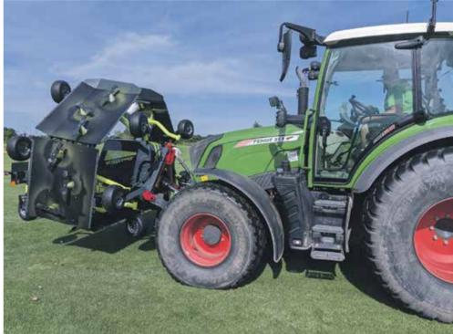
and quiet. The large wheels and clever deck linking system ensure good contour following and enable high mowing speeds.
