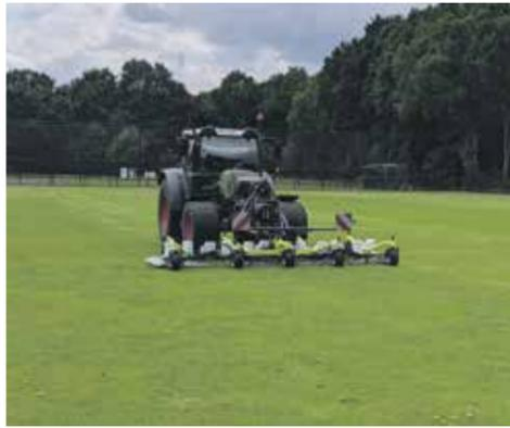
cutting decks. The forward position provides excellent visibility and comfort for the tractor operator.
