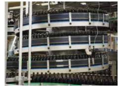
Ministellation for the elevation of filled glass bottles at the OeTTINGER brewery in Mönchengladbach. This is the first of our new vertical mass-flow conveyor system. It is a stainless steel spiral conveyor, fitted the new single track design complete with the recently developed TPJ4 slat.
