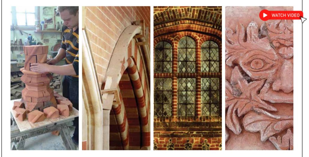
Bulmer bricks are made from the finest London Clays, dug from our seams almost continually since Tudor times. All Bulmer bricks are hand made, using traditional methods of making, drying and are fired in a coal burning, down draught kiln. This helps to give the distinctive finish that blends so well with the originals. The process takes time – something to consider at the project planning stage.
