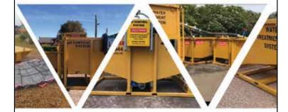
SETTLE & RETAIN SOLIDS FLOCCULATION & LAMELLA NEUTRALISE & CONTROL PH REMOTELY MONITOR PH & TSS
