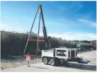
treatment systems. All our boreholes are constructed using the cable-tool percussion method - preferred by the Environment Agency (EA) when drilling the chalk aquifer - and are logged with the BGS. Our underpinning ethic is that we want to protect the aquifers from which we make our living.
