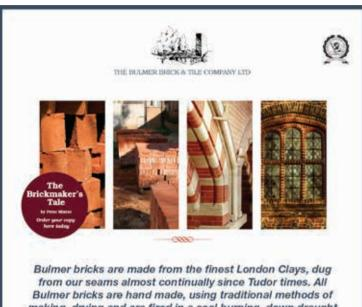
making, drying and are fired in a coal burning, down draught kiln. We are a small family business continuing the traditions of brickmaking on this site dating back to the Middle Ages.
