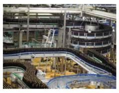
mbaFlex is proud to present our lates Ainstallation for the elevation of filled glass bottles at the OeTTINGER brewery in Mönchengladbach. This is the first of our new vertical mass-flow conveyor system. It is a stainless steel spiral conveyor, fitted the new single track design complete with the recently developed TPJ4
